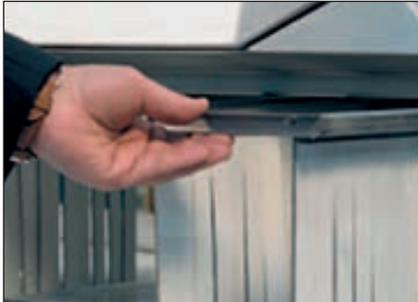
The **belt length** is entirely configurable, based on customer requirements and available space. Thanks to the use of a new **motor-driven drum system**, the length can be reduced to 1 m and the belt combined with existing belts, without difficulties caused by the size of normal external motors.
